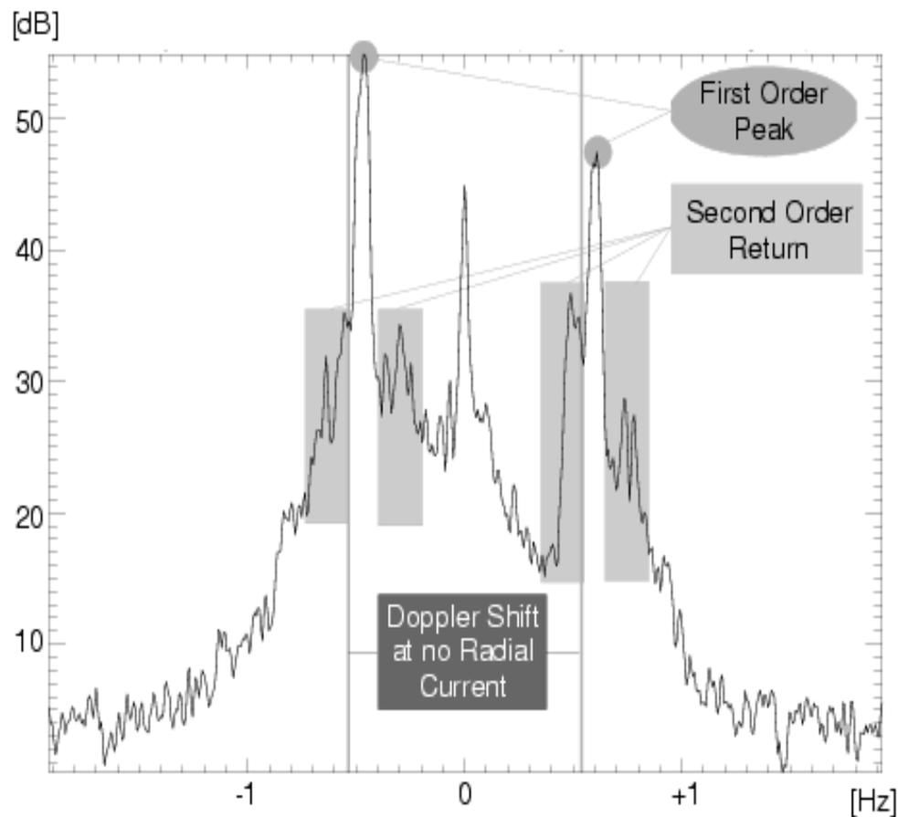
**Significant wave height (SWH)** is derived from scaled ratio of 2<sup>nd</sup> order to 1<sup>st</sup> order peaks from a single radar site.
